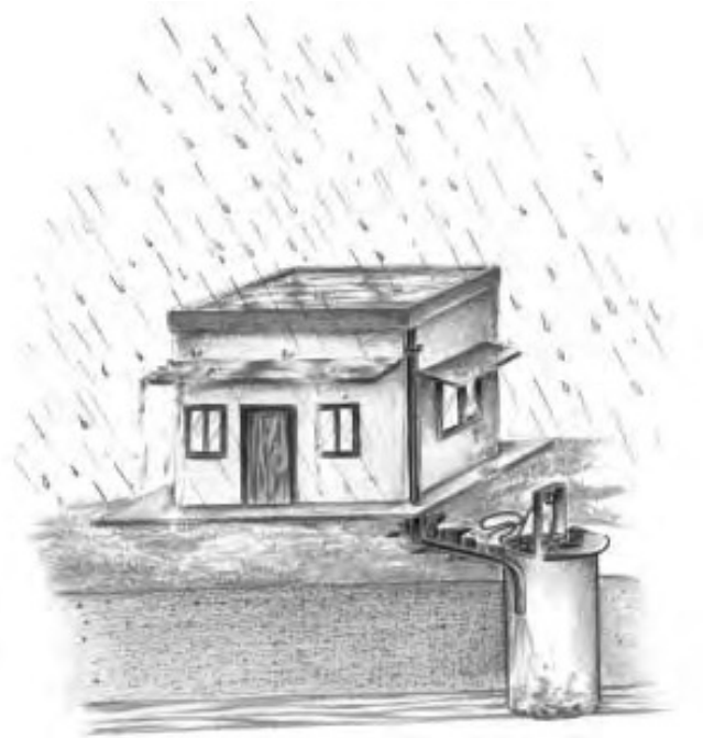
(b) Recharge through Abandoned Dugwell
