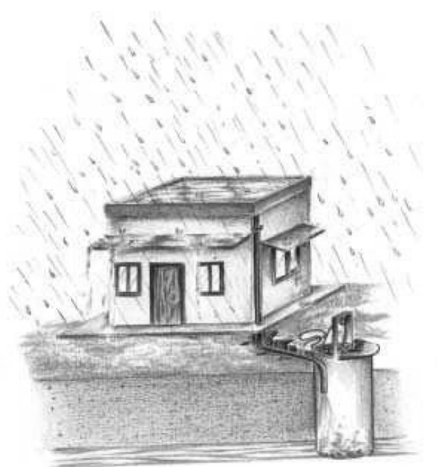
(b) Recharge through Abandoned Dugwell
