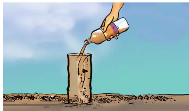
Fig. 9.5 Measuring rate of percolation
