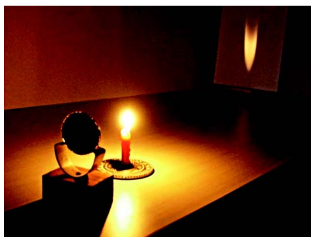
Fig. 15.15 Real images formed by a concave mirror
