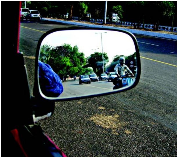
Fig. 15.20 Convex mirror as side view mirror
