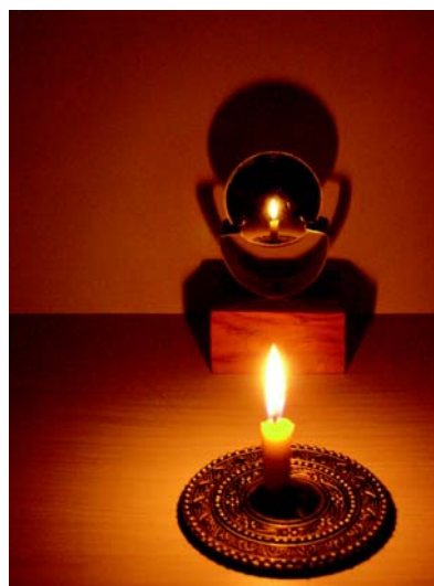
Fig. 15.19 Image formed by a convex mirror
