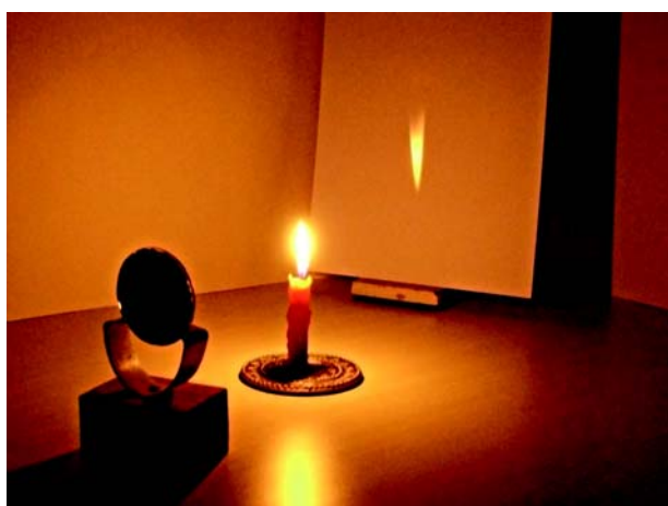
Fig. 15.15 Real images formed by a concave mirror
