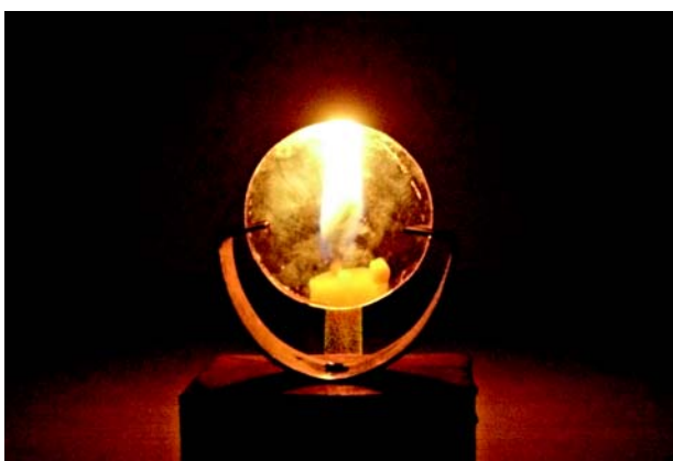
Fig. 15.26 Virtual image formed by the convex lens
