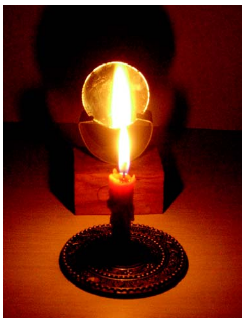
Fig. 15.16 Virtual image formed by a concave mirror
