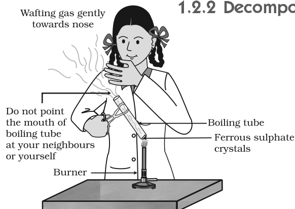
Figure 1.4 Correct way of heating the boiling tube containing crystals of ferrous sulphate and of smelling the odour
